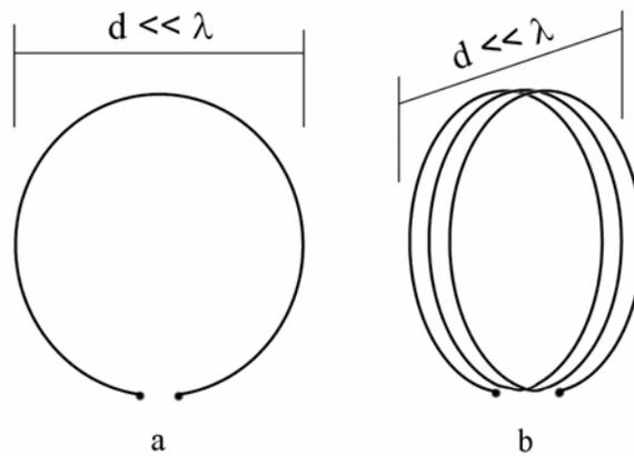
Fig. 3. Loop antenna (a) and a few turns coil (b).
